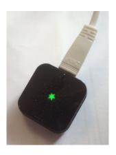
2.3 With a paper clip or similar gently push the clip through the reset hold and press until the green light goes out.
